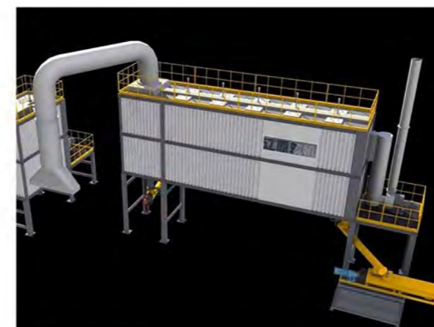
Dust Collecting System: one gravitational dust collector, two bag-house dust collectors
