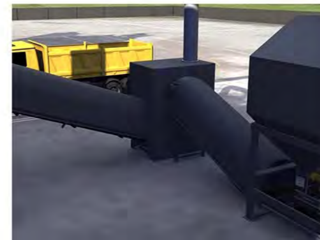
Enclosed Belt Conveyor
